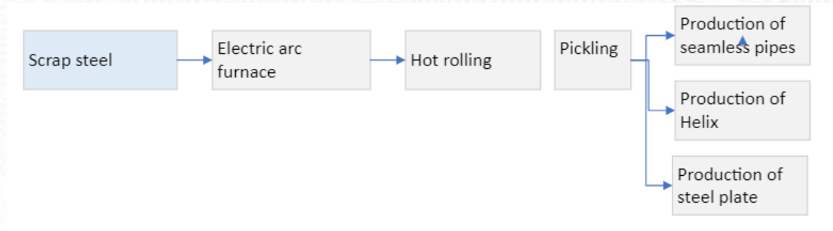
Figure 3: Steel Production Process Via Electric Arc Furnace
